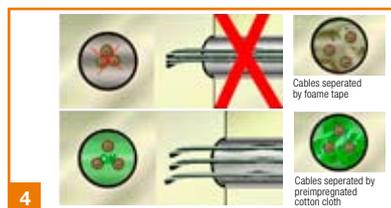
Use foam tape or cotton cloth as suitable barrier and to separate the cables from each other.
