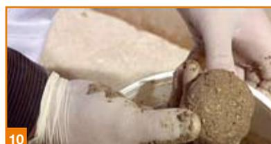
To check for appropriate malleability, the mortar should be moulded to a ball shape without falling apart.
